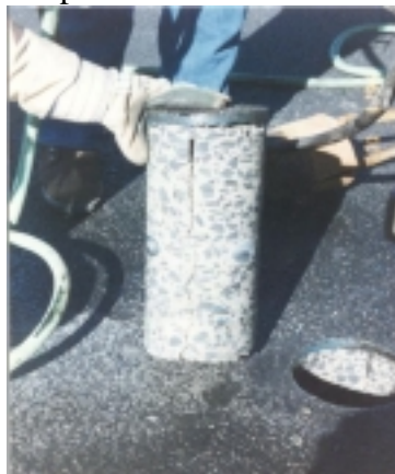
Figure 2. A core specimen of a thin AR-ACFC on PCCP.
